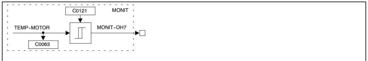
Fig. 2-155 Monitoring of the motor temperature, with adjustable threshold (OH7)
