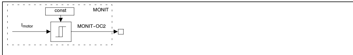
Fig. 2-148 Earth-fault monitoring (OC2)
