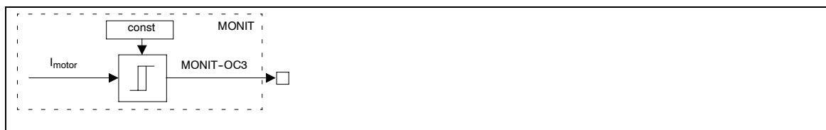
Fig. 2-149 Overload during acceleration or deceleration OC3
