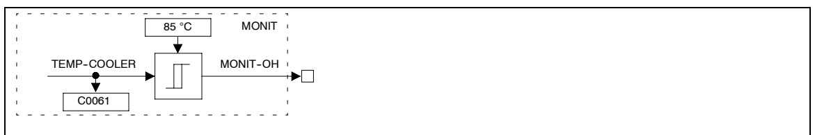
Monitoring of the heatsink temperature, with fixed threshold (OH)
