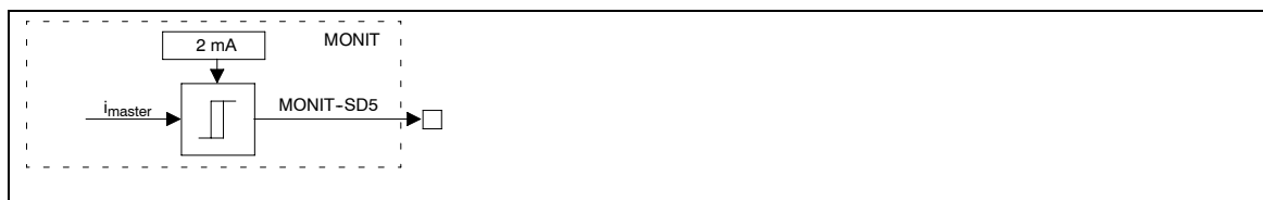
Monitoring of the encoder at X6/1, X6/2 (Sd5)
